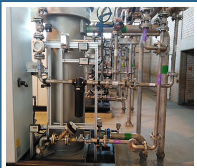
Figure 2: Ozone Generator Vessel containing Electrodes
