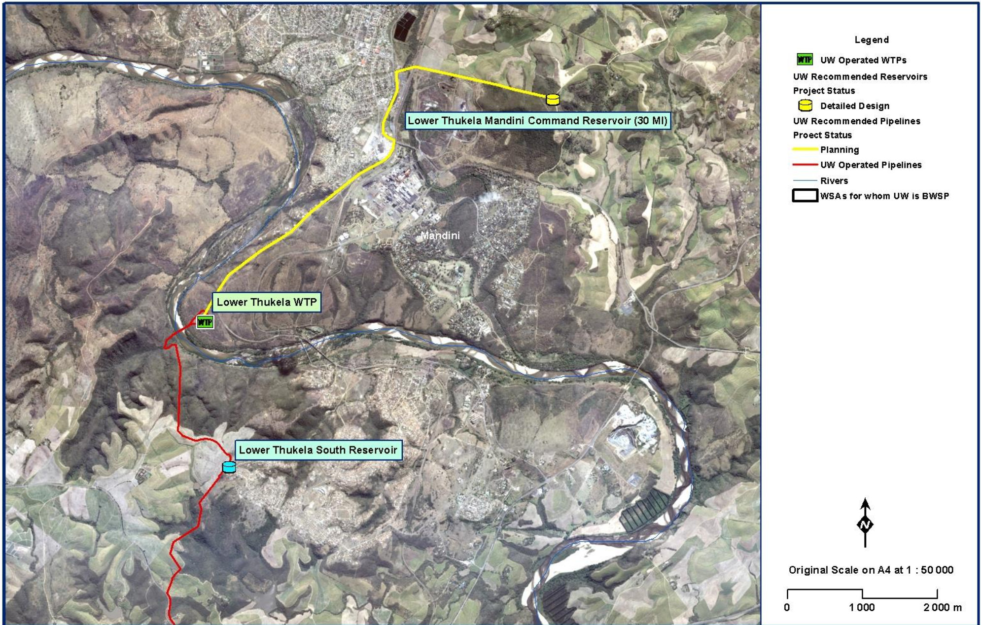
Figure 12.43 Lower uThukela Bulk Water Supply Scheme – Phase 2.
