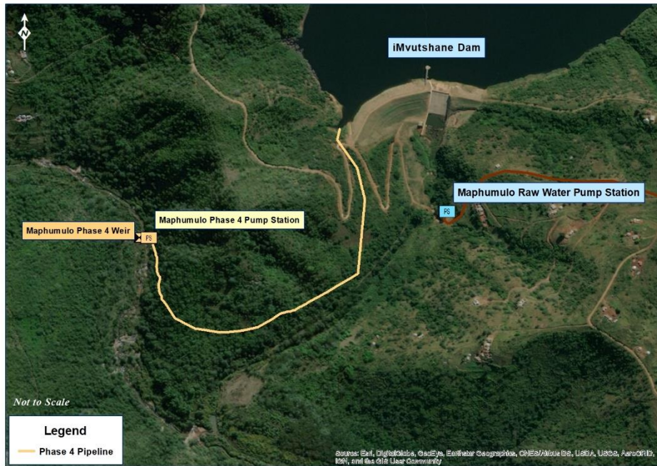
Figure 12.14 Locality map showing the proposed Hlimbitwa River weir pump station in relation to iMvutshane Dam.
